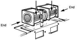
7. Guide wires into duct while placing blower unit back into opening.
